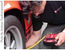
Keeping track of tire pressures and temperatures is crucial when trying to get the best out of the car's set-up.
