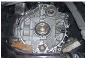
The solution is to install direct oil injection to the IMS bearing using the engine's own pressurized oil. The M96/ M97 engines have several unused high-pressure oil ports already built into the block, so it is very easy to tap into one of them. A high-pressure stainless-steel braided oil line is
