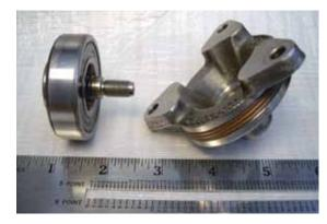
This is an OEM single-row bearing which just came off a Carrera 996. You can see how the bearing is sealed. There is no way this bearing would get proper lubrication under the conditions where it is installed. This bearing was extracted as it had just begun to fail. The owner was very lucky we caught it in time.
