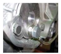
A small notch needs to be cut into the edge of the bell housing to allow for the routing of the oil hose. When this new flange is installed, it is recommended that the existing IMS bearing be replaced with either a new ceramic-ball bearing or a new OEM all steel bearing.
