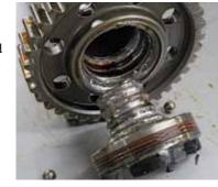
All of the three IMS bearings Porsche installed in the M96 and M97 engines have been known to fail.
