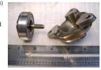
but for model year 2009 the factory introduced a brand new engine, the MA1, which does not have an intermediate shaft (IMS) nor the IMS bearing. Cars that are driven regularly and driven hard have fewer IMS bearing failures than those that are babied and sit in a garage or are not tracked or driven spiritedly. If the IMS bearing fails the most likely result is catastrophic engine failure.
