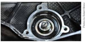
MS bearing with seal and (below) without
