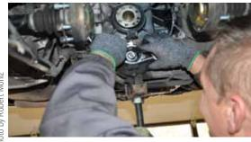
Zoran removing bearing cap
