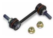
The first to go are usually the drop-links which can cause quite a rattle when driving over pavers or irregular pavement. Most of these parts are difficult to diagnose
