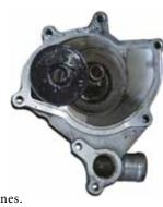
When this happens the pump is no longer balanced and starts to destroy its seal and bearing. When the pump fails, all coolant will be lost, rendering the car un-drivable. The water pump is more expensive than the previous wear items, costing around \$300 for the part, three to four hours labour plus materials, such as gaskets, coolant concentrate, distilled water, etc.
